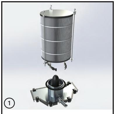
Position Filter Assembly over the cylinder (1 rod facing front, space between 2 rods facing towards back, strap unclasped) and pull cylinder braces outward while lowering to clear halo guard.
