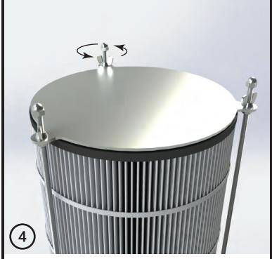
Once Filter Assembly is attached, adjust wingnuts at top to secure a stable fit. Be careful to not tighten down top cover too much as it will begin to warp the pleats of the filter cartridge.
