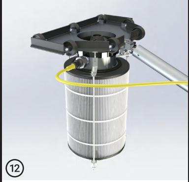
To remove filter cartridge, place upside-down on deck. Disconnect battery cable and remove Bottom Feeder unit. We recommend rinsing inside pleats of filter after each use with garden hose equipped with pressure nozzle.
