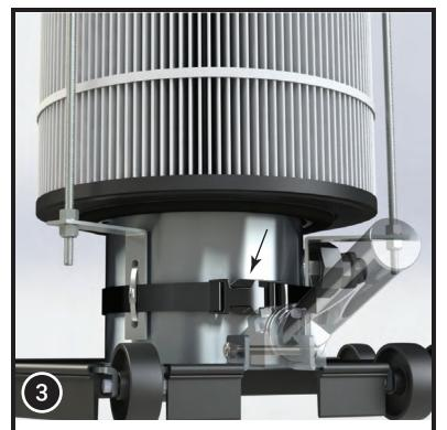
Latch the clips on the cylinder brace strap to secure Filter Assembly to The Bottom Feeder. Check strap fit and make sure there is a snug fit. Adjust strap if necessary.
