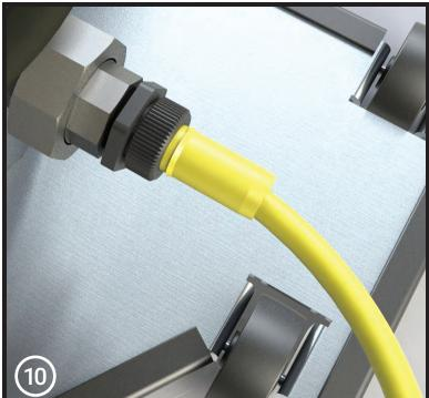
Finger tighten the lock nut on the battery connector onto the receptacle on head of unit. Do not run dry more than a minute.
